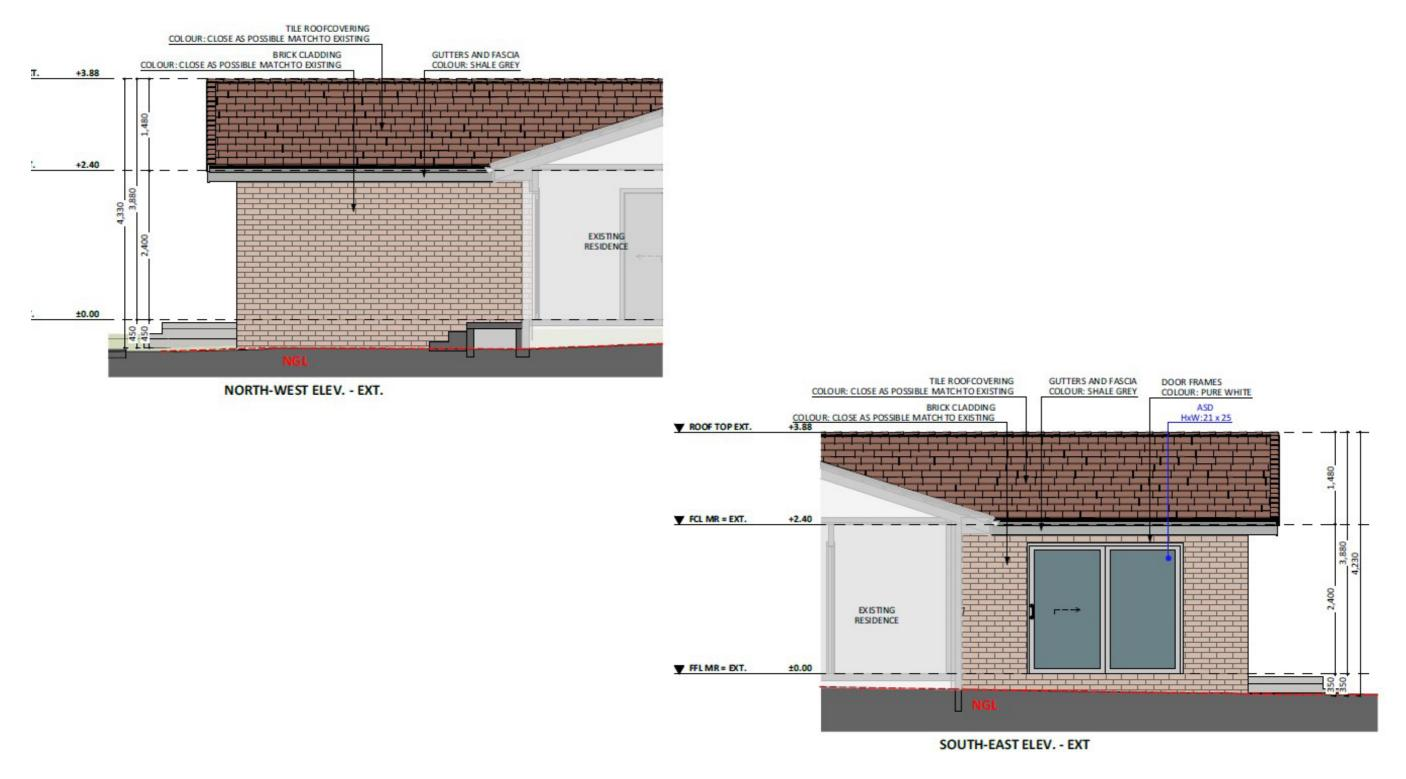
Disclaimer: based on the alternative roof designs and roof covering that you may select and the profile of your block, these elevations are subject to potential change.
